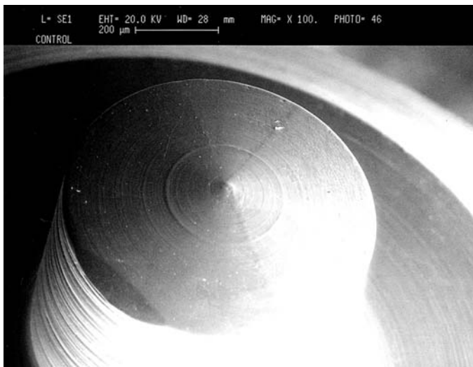
51E2657 Poppet sealing surface viewed with Lockheed Martin SEM. Poppet never installed.
