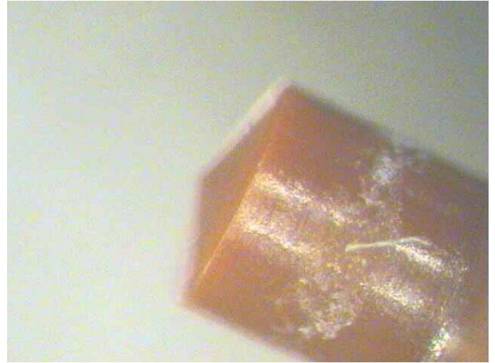
51E265 SN007 Poppet tip showing white residue (aluminum silicate)
