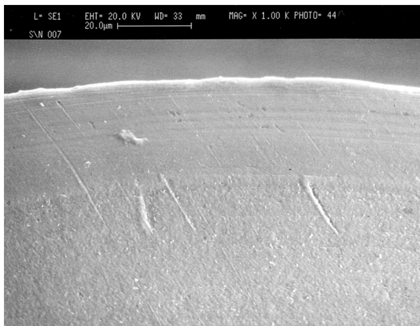
51E265 SN007 Poppet sealing surface viewed with Lockheed Martin SEM. Note scratches.
