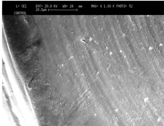
51E265 Poppet sealing surface viewed with Lockheed Martin SEM. Note localized high and low spots and scratches. Poppet never installed.
