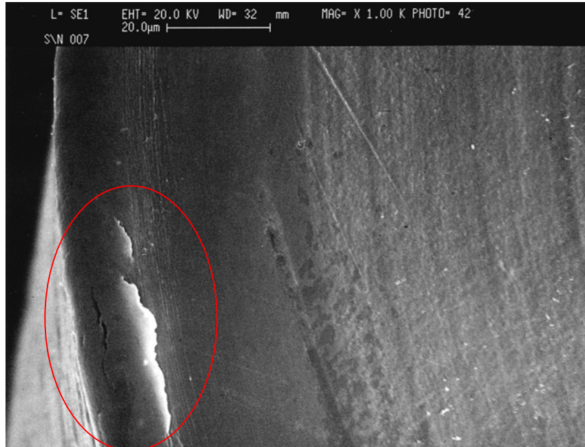
51E265 SN007 Poppet sealing surface viewed with Lockheed Martin SEM. Note burr near sealing edge.
